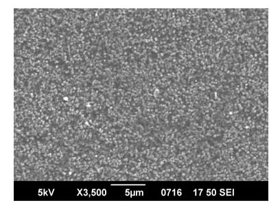
As the growth temperature increases to 550 ° C, surface diffusion is activated, the surface morphology becomes flattened, and columnar grains of uniform size and shape are formed.
