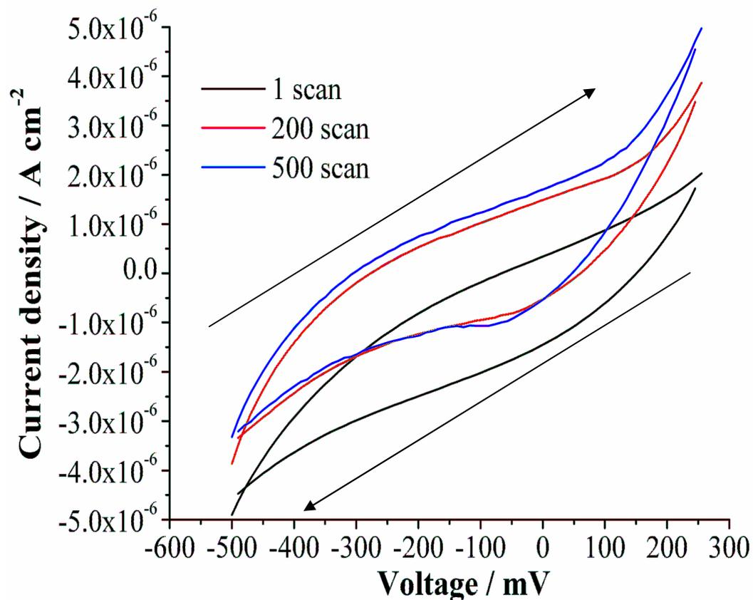
□ The current density increases from 1st to 200th cycle and shows no appearance of degradation after 200 cycles,
