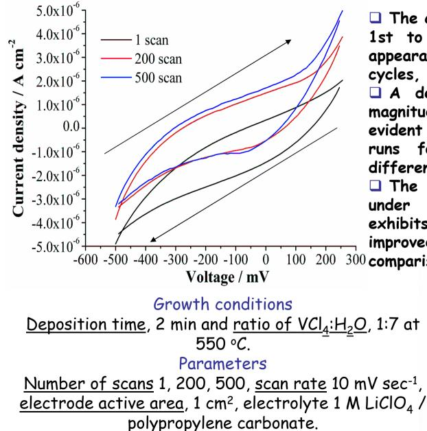
□ The current density increases from 1st to 200th cycle and shows no appearance of degradation after 200 cycles,
