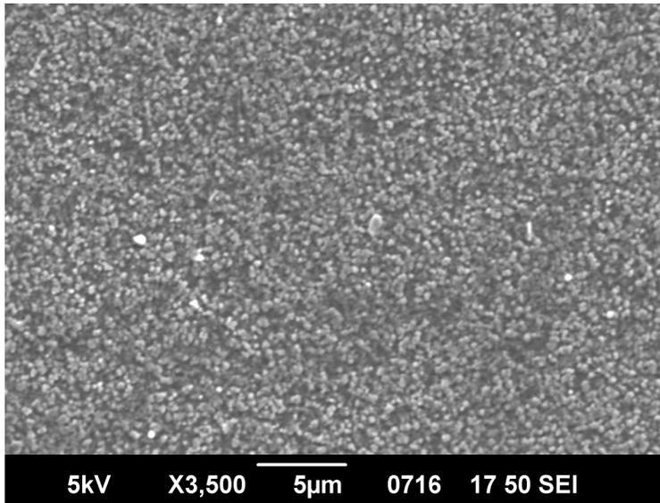
As the growth temperature increases to  $550\text{ }^{\circ}\text{C}$ , surface diffusion is activated, the surface morphology becomes flattened, and columnar grains of uniform size and shape are formed.
