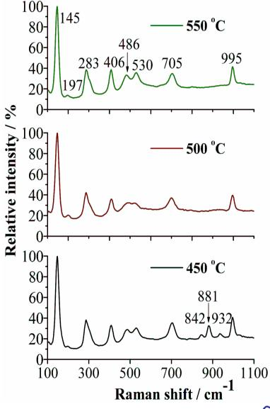
✓ Only a single phase of  $V_2O_5$  was detected apart from the samples grown at 450 °C,
