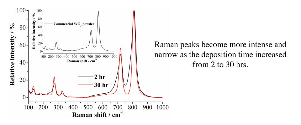
**Growth conditions** <u>Deposition time</u>, 2 and 30 hr, <u>Deposition temperature</u>, 95 °C <u>Precursor</u>, 0.3 M NaOH with 0.0021 M WO<sub>3</sub>
