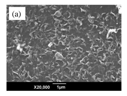
Wall-like structures are formed with a relatively porous morphology.
