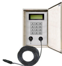
Figure 4: Photograph of the System Control Unit.
