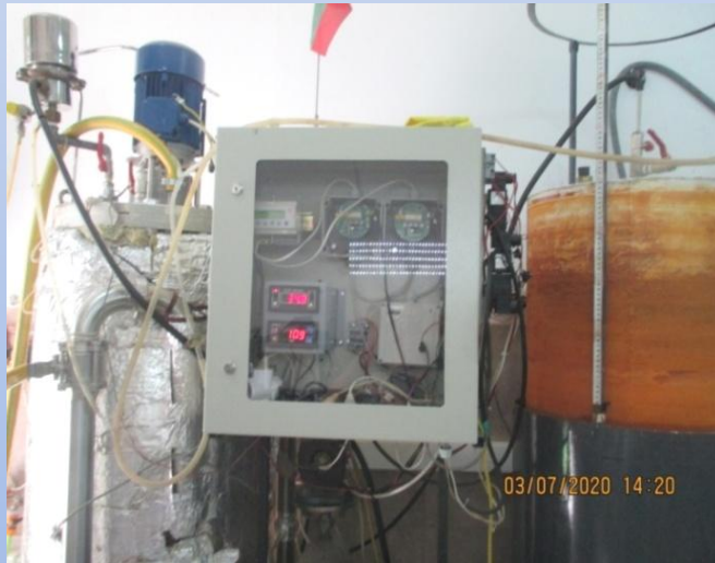
Fig. 3. Different view of the pilot-scale ABR with automatic control system:
