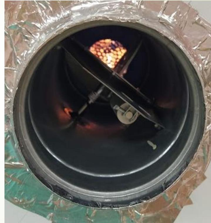
The grid, placed in the device to linearize the air flow before the measurement by the pressure sensor.
