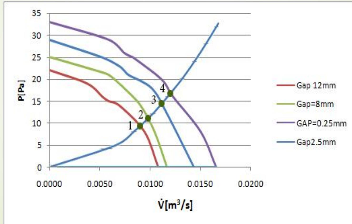
Overlay of graphs of fan's efficiency for different gap values 0.25mm, 2.5mm, 8 mm dhe 12 mm.
