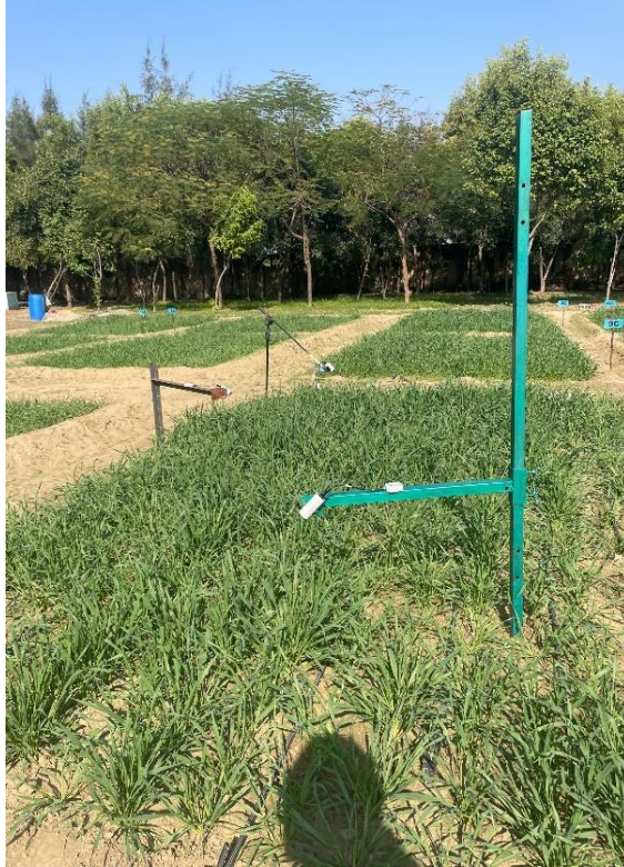
Image. Crop temperature Data collection through IRT
