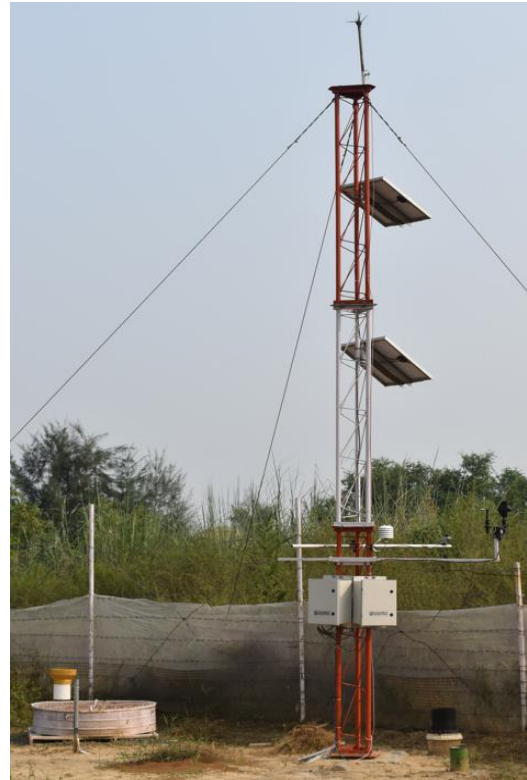
Image. Automatic weather station installed at the field laboratory
