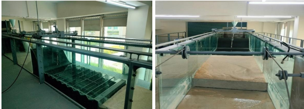
Images: Recirculating indoor experimental flume
