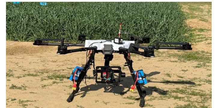
Image. Hyperspectral and multi spectral camera mounted on drone
