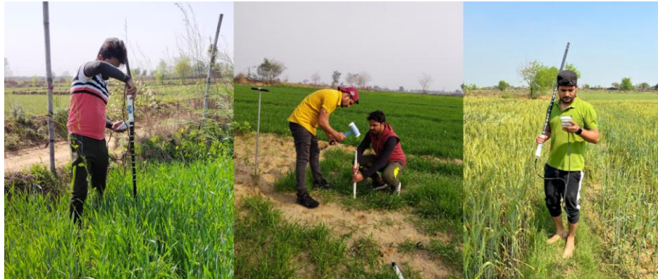
Image: Installation of access tubes and soil moisture data collection
