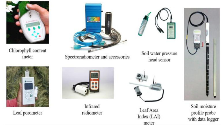
Image. Different research grade equipment used for the monitoring of soil and crop parameters
